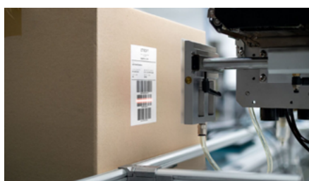
Application of labels up to 180 mm wide
